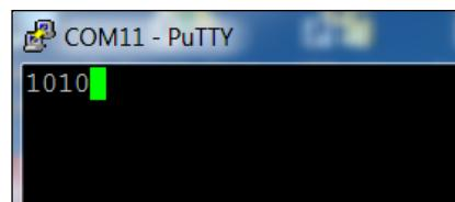
Now, if your system is not working, there are a couple of ways to try and determine what is going wrong. First and foremost, make sure Arduino is turned on and is executing the correct code. Second, check to see that characters are being typed in the PuTTY window. Third, check the baud rate of the PuTTY window. If this is too high, you will see characters come through the system, but they will not be interpreted correctly on Arduino.
