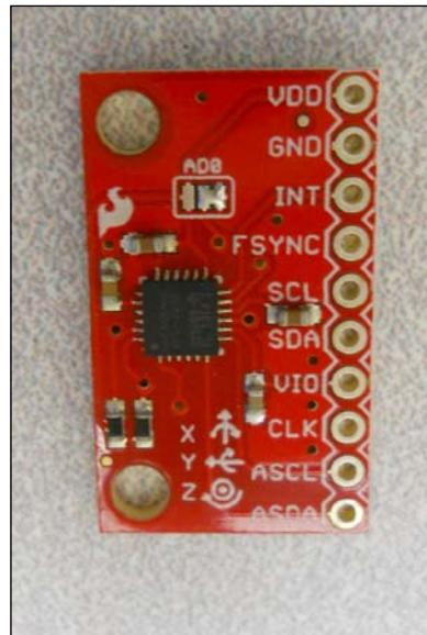
The interface to the board is quite simple, with only one issue. One of the ways to connect this particular chip is to solder header pins to the board to connect the jumper wires to Arduino. You can purchase these at [sparkfun.com](http://sparkfun.com) as well; just search for the Arduino stackable header, 8-pin version. Once the header is soldered, the device will look as follows:
