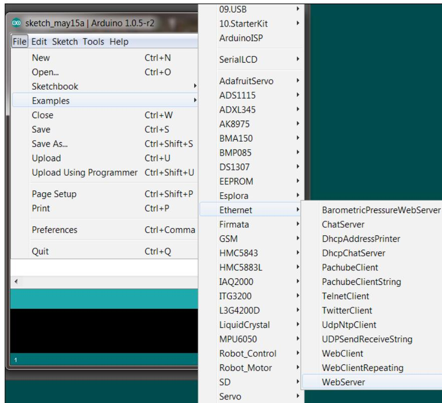
Using a web server will allow you to access your Arduino via the LAN cable that will be connected to your ROV from a web browser on a computer at the surface. To connect with the device, you'll need to set the appropriate address for the Arduino web page.
