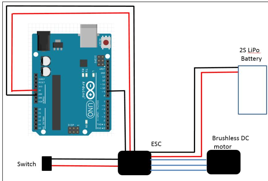
For details on the connection between the ESC and brushless DC motor, check your ESC documentation. Now that you've connected your motor, a simple sketch to control the motor is shown in the following screenshot:
