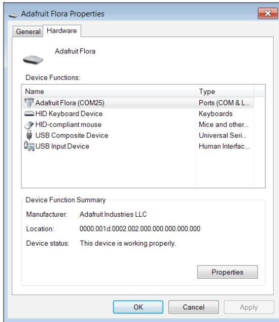
Note the device COM port; in this case, it is COM25. Now, you should open the Adafruit Arduino IDE by going to the directory where you unzipped the files and select the Arduino IDE. Just a note, since I often use both types of Arduino devices, I have a separate directory for the standard Arduino IDE and a different location for the Adafruit Arduino IDE. To open the Adafruit Arduino IDE, I go to the file browser and select the Arduino IDE executable:
