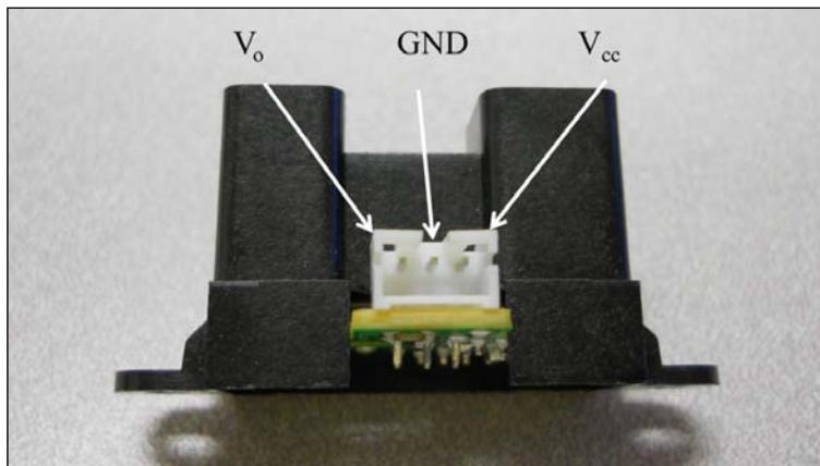
One of the challenges of making this connection is that the female-to-male connection jumpers are too big to connect directly to the sensor. You'll want to order the three-wire cable with connectors with the sensor, and then you can make the connections between this cable and your Arduino device using the male-to-male jumper wires. Once the pins are connected, you are ready to access the sensor via the Arduino IDE.
