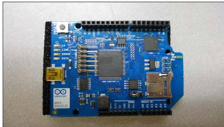
Place the shield onto the Arduino Uno and you are ready to connect to a wireless network.
