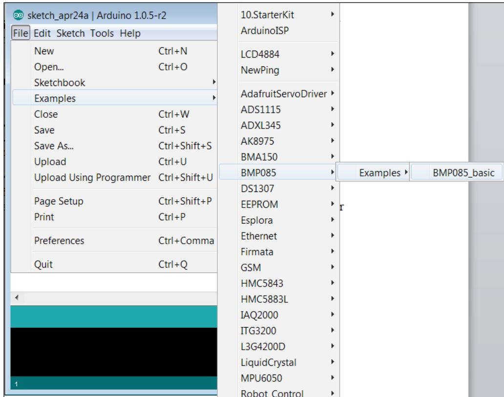
3. You should now set the Serial Monitor baud rate to 38400 if you haven't already done so, as this is the baud rate set by the example program. Now, you can upload the sketch of Arduino, and when you open the Serial Monitor, you should see something similar to the following screenshot:
