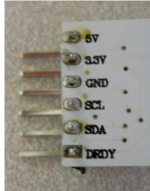
The following are the connections that you'll need to make between Arduino and the device:
