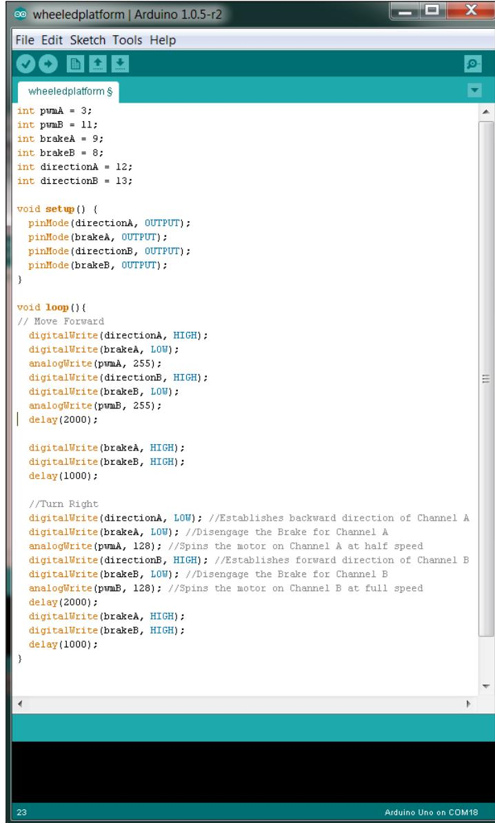
The screenshot shows the Arduino IDE interface with the title bar "wheeledplatform | Arduino 1.0.5-r2". The code editor contains the following C++ code for controlling two DC motors via a shield:
