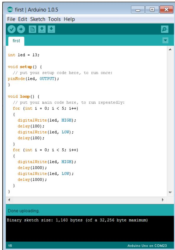
The screenshot shows the Arduino IDE interface with a sketch titled "first". The code contains two `for` loops. The first loop runs 5 times, alternating LED states every 100ms. The second loop runs 5 times, alternating LED states every 1000ms. The code is as follows:
