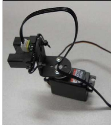
You'll need to connect both the IR sensor (as described earlier in this chapter) as well as the servo to Arduino (as explained in *Chapter 7, Controlling Servos with Arduino*).
