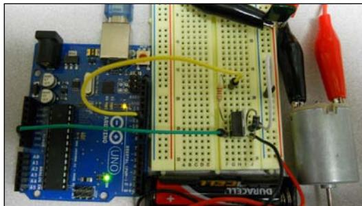
Now, you can start the Arduino IDE and enter a program to send a control signal to the DC motor.
