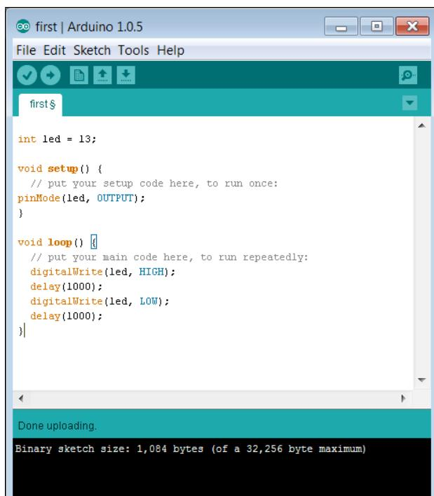
The screenshot shows the Arduino IDE interface with a sketch titled "first". The code defines a variable `led` at pin 13, sets up pin 13 as an output in the `setup()` function, and then enters a `loop()` function where it alternates between `digitalWrite(led, HIGH);` and `digitalWrite(led, LOW);` every 1000 milliseconds using `delay(1000);`. The status bar at the bottom indicates "Done uploading." and "Binary sketch size: 1,084 bytes (of a 32,256 byte maximum)".
