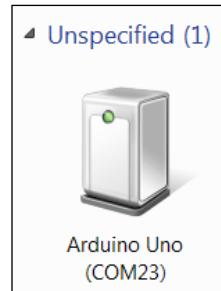
In this case, the device is connected to COM port 23. Note down the COM port Arduino is connected to as you'll need that in a minute. If you are using an Apple Mac or Linux machine, follow the instructions at [arduino.cc/en/Guide/MacOSX](http://arduino.cc/en/Guide/MacOSX) for Mac and [playground.arduino.cc/Learning/Linux](http://playground.arduino.cc/Learning/Linux) for Linux on how to determine your USB port connection.
