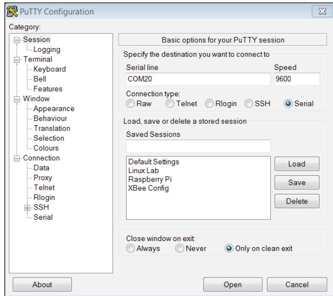
2. Configure the terminal window and set the following parameters:
