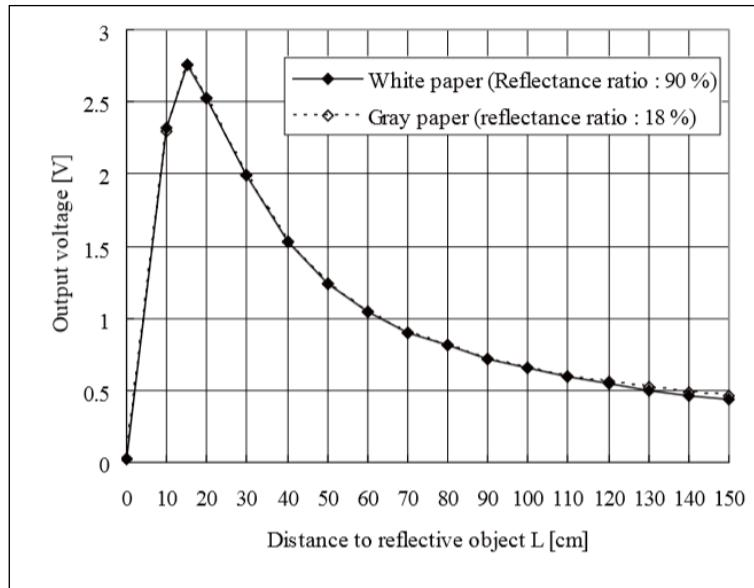
There are two parts to the curve. The first is the distance up to about 15 centimeters and then the distance from 15 centimeters to 150 centimeters. This simple example ignores distances closer than 15 centimeters, and models the distance from 15 centimeters and out as a decaying exponential with the following form:
