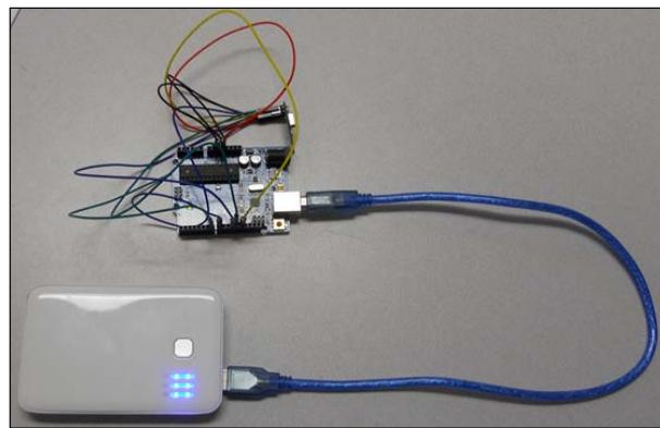
The LED on the receive Arduino should be flashing, indicating that the two Arduinos are communicating.
