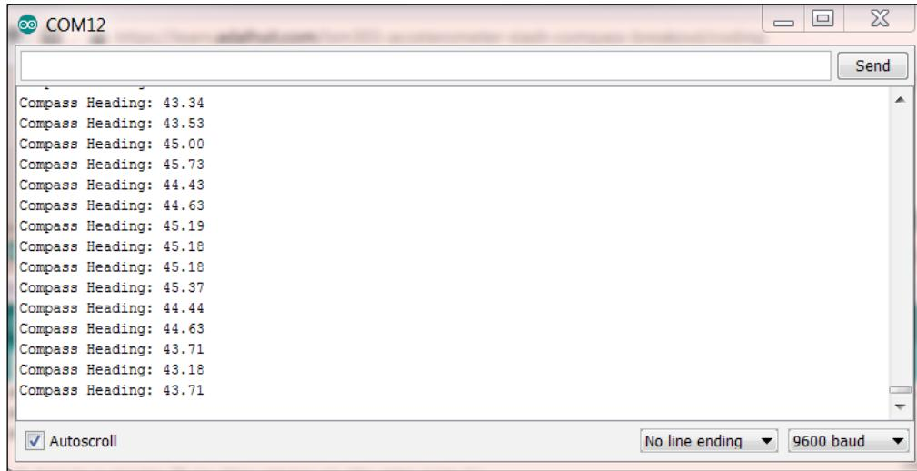
Now, you have access to `Compass Heading`. The final step is to merge the NeoPixel code with the `Compass Heading` code. The following is a simple example that changes color based on the direction:
