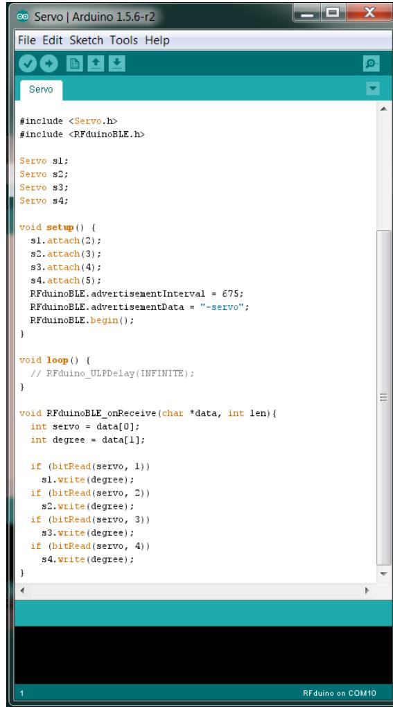
The screenshot shows the Arduino IDE interface with a sketch named "Servo". The code uses the RFduinoBLE library to control four servos (s1-s4) via Bluetooth. It initializes the servos and sets up the RFduinoBLE module with an advertisement interval of 675 ms and data "-servo". The loop reads data from the Bluetooth connection and writes the received degree value to each servo's position.
