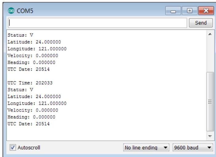
These are the GPS readings from the device. As noted in the previous section, **Status** tells you whether or not your device is locked to enough satellites. In this case, **V** indicates that our device is not. You may need to go outside a building to connect with enough satellites to get a valid reading. A valid reading would look like the following screenshot:
