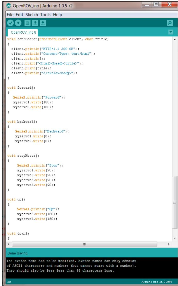
The screenshot shows the Arduino IDE interface with the sketch named "OpenROV\_arduino". The code is as follows:
