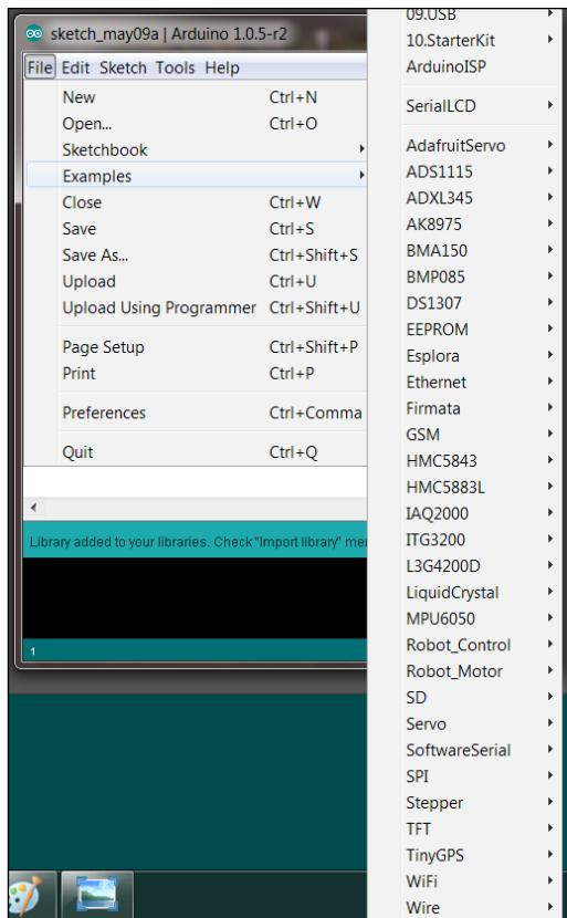
These are all very useful examples. Just to make sure that your shield works, you can select **ScanNetworks**. Run this program and open **Serial Monitor**. This program scans for available networks and should show a set of networks that are possible to connect to.
