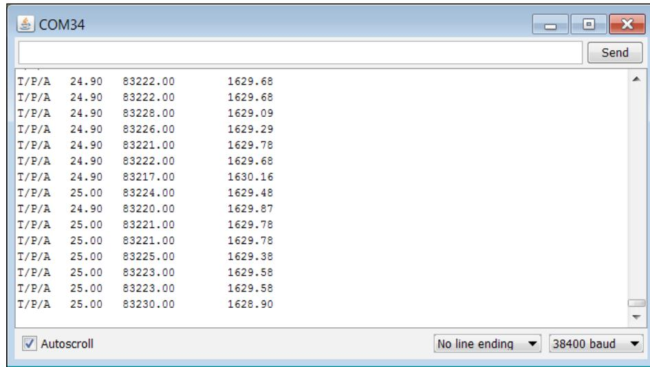
You can see not only the altitude, but the temperature and pressure as well. Now, this altitude is not an absolute value, but a relative one. It will change with a change in weather, as the barometric pressure is dependent on weather pattern changes. This particular reading is, therefore, really only useful when you want to measure the relative changes in altitude, for example, when you want to know how far your flying project has either gone up or done from a reference position.
