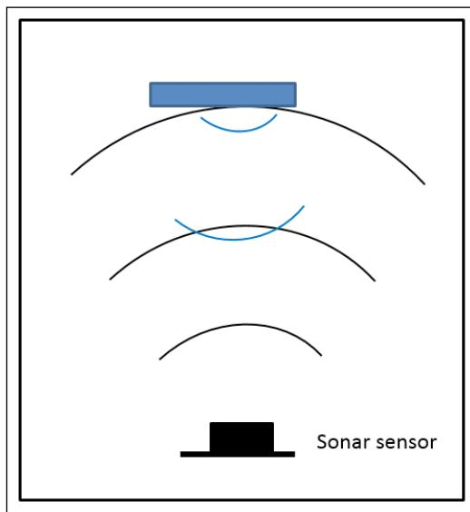
The sensor measures the returning sound waves. It uses the time difference between when the sound wave was sent out and when it returns to measure the distance to the object.
