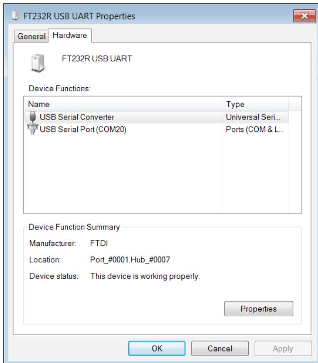
Note that the device is connected to the **COM20** serial port. We'll use this to communicate with the device and configure it. You can use any terminal emulator program; I like to use PuTTY. If you don't have PuTTY, you can download it from [www.chiark.greenend.org.uk/~sgtatham/putty/download.html](http://www.chiark.greenend.org.uk/~sgtatham/putty/download.html). This will provide an executable file that you can run to talk with and configure the devices.
