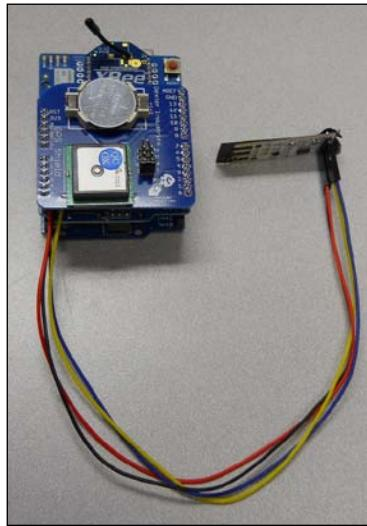
The wind sensor is connected to the holes available on the Wireless SD shield. You'll also need to add the servo control, but now, you have all the capabilities you need to build your Arduino-controlled sailing vessel. However, Arduino is not limited to just sailing above the water. Let's see how you can build a robot that can go under water.
