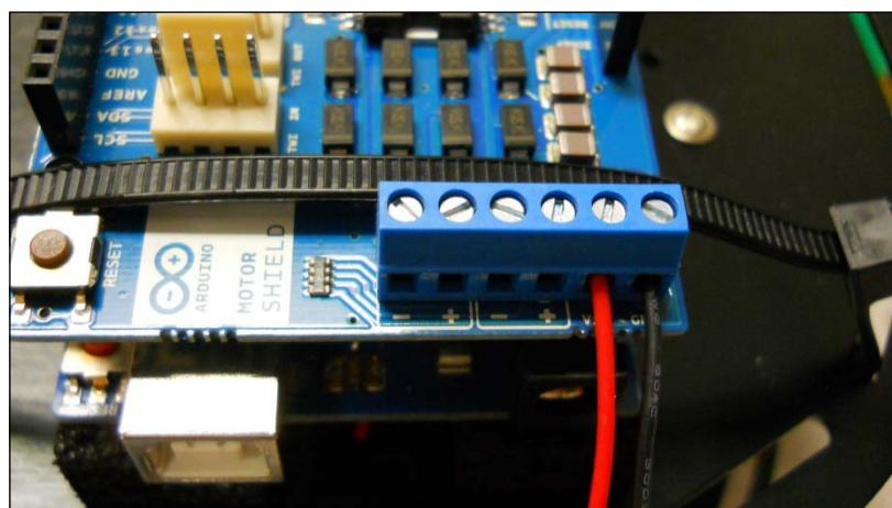
Now, you need to connect the motor shield to the motors. If you don't want to solder wires to the motors, you can use the alligator clip wires as shown in the following figure:
