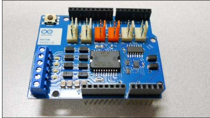
Specifically, you'll care most about the connections on the front corner of the shield, which is where you will connect the two DC motors. This is shown in the following figure:
