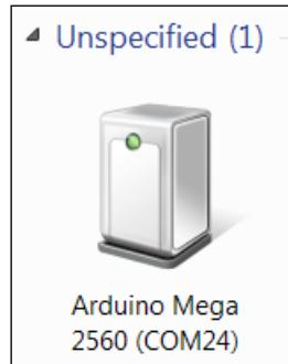
Note that in this case, Mega is connected to COM port 24. The port that Arduino will be connected to is selected by the computer and is not the same for all Arduinos. The only difference between the instructions for using Mega and Uno is that you will need to set the correct board type for Mega. To do this, navigate to **Tools | Board | Arduino Mega 2560 or Mega ADK** as shown in the following screenshot:
