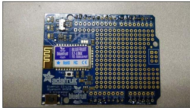
Unfortunately, you'll need to solder header pins onto the shield to mount it on your Arduino, but then, you'll need no additional connections. You'll also need a USB module if you want to communicate with your PC. The following is an image of an adapter that is also available at [www.adafruit.com](http://www.adafruit.com):
