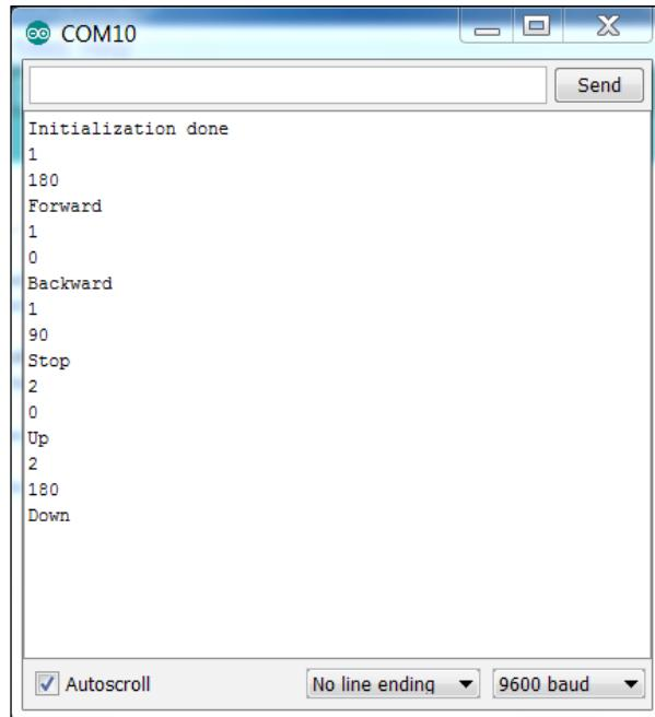
If your motors are connected to the control pins, as covered earlier in the chapter, your motors should be ready to drive your ROV up, down, backward, forward, or stop all motors. You may have to adjust the settings based on the direction of your motors' spin and also the desired speed.
