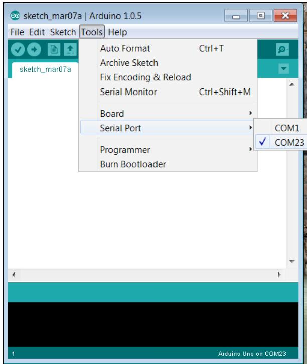
The IDE should now indicate that you are using the Arduino Uno on COM23 in the lower-right corner of the IDE, as seen in the preceding screenshot.
