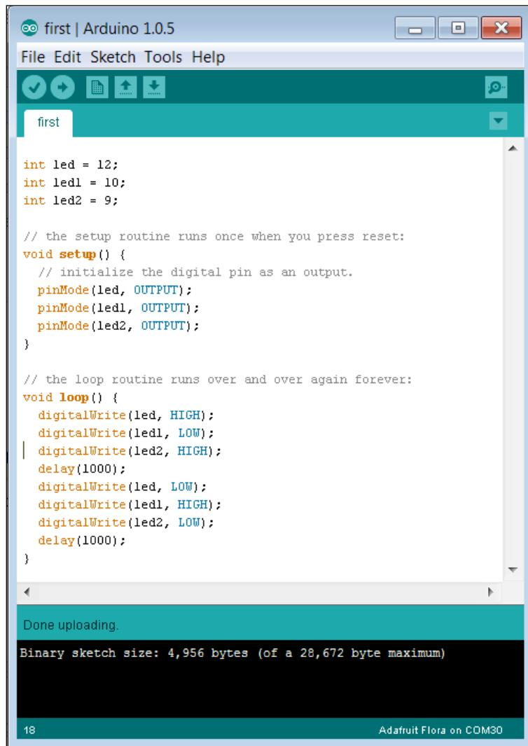
The screenshot shows the Arduino IDE interface with a sketch titled "first". The code initializes three pins (led, led1, led2) as outputs and sets up a loop where each pin alternates between HIGH and LOW states every second. The upload process is completed, indicating a binary sketch size of 4,956 bytes.
