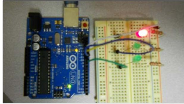
You'll need to add a similar bit of code to get the LEDs connected to pins 12 and 11. Add the code snippet that can be seen in the following screenshot to the sketch on the Arduino IDE:
