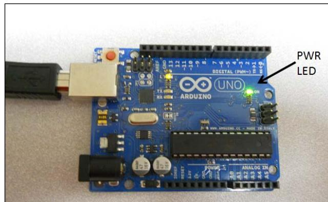
The Arduino Uno is also preloaded with a simple blink program; the yellow LED should also be turning on and off every second. The Mega will look very similar to the Arduino Uno.
