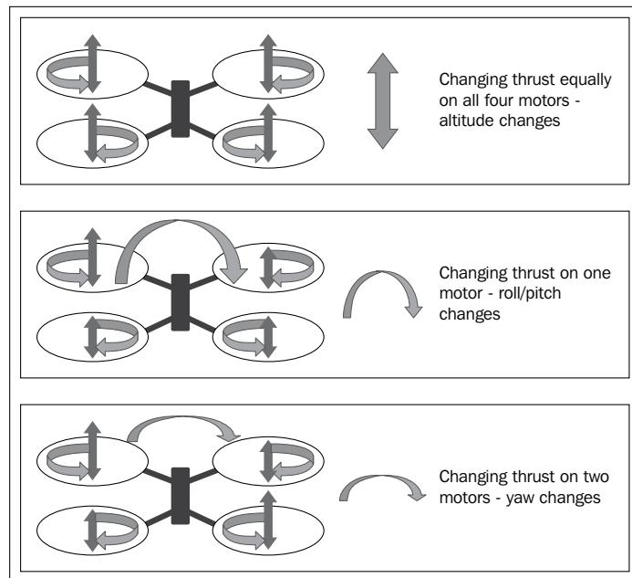
As you can see, controlling the relative speeds of the four motors allows you to control the various ways in which the device can change position. To move forward, or really in any direction, we would combine a change in roll/pitch with a change in thrust so that instead of going up, the device would move forward, as shown in the following diagram:
