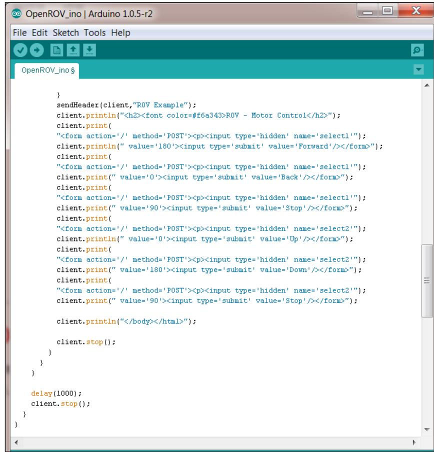
The screenshot shows the Arduino IDE interface with the sketch named "OpenROV\_ino". The code is written in C++ and uses the Arduino API for network communication via a WiFi shield. It includes functions for sending HTTP headers, printing HTML forms for motor control, and handling POST requests to change the motor speeds. The code also includes a delay of 1000ms and a call to client.stop() at the end of the main loop.
