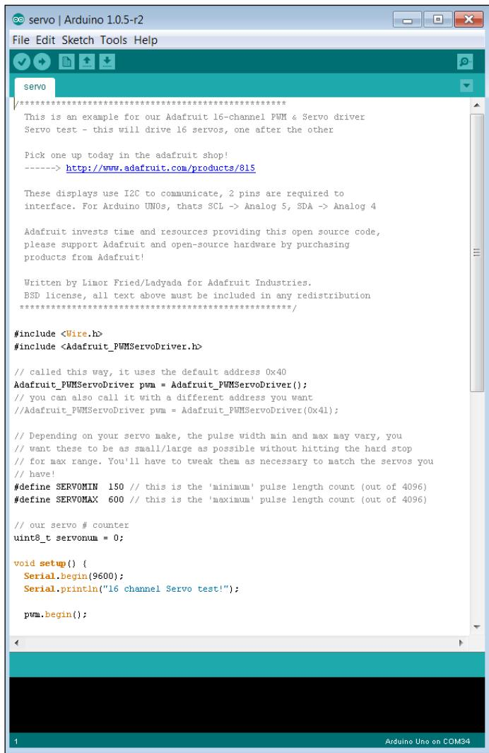
The screenshot shows the Arduino IDE interface with the title bar "servo | Arduino 1.0.5-r2". The menu bar includes File, Edit, Sketch, Tools, and Help. The toolbar has icons for upload, refresh, and other functions. The code editor contains the following C++ code for controlling servos:
