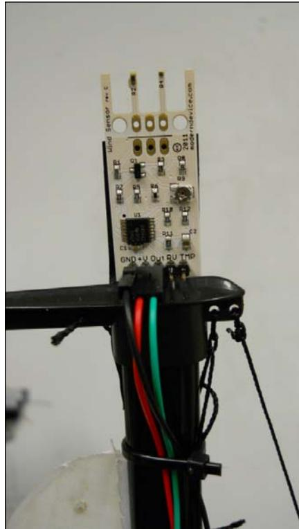
To add this to your system, you'll also need a way to take the analog input from the sensor and send it to Arduino. Notice that the device has three connections that you'll be using: GND, +V, and Out. Connect your Arduino to the wind sensor using the following connections:
