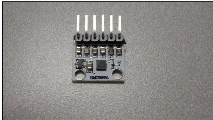
This type of digital compass uses magnetic sensors to discover the earth's magnetic field. The output of these sensors is then made accessible to the outside world through a set of registers that allow the user to set things such as the sample rate and continuous or single sampling. The x, y, and z directions are output using registers as well.
