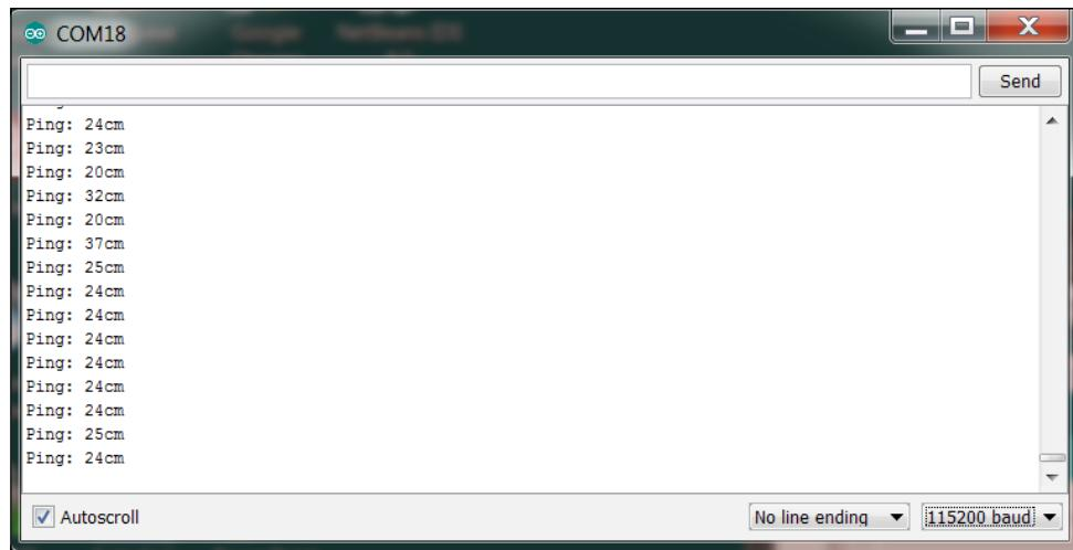
You can now measure the distance to an object using your sonar sensor.
