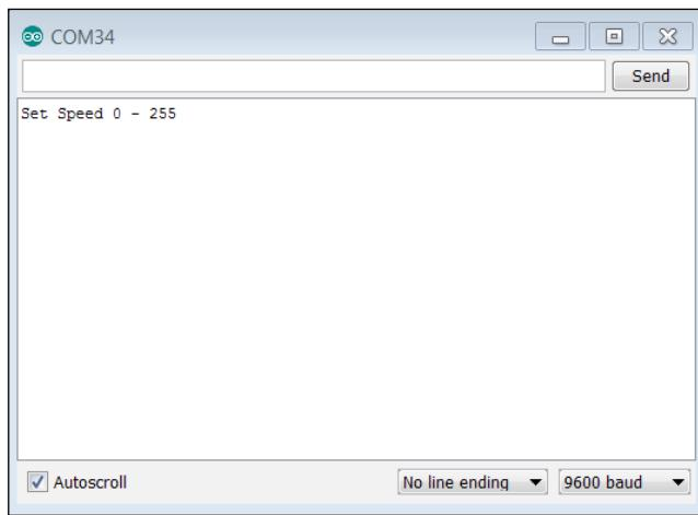
2. Enter a value, for example, 255, and then click on **Send**. Your motor should speed up. Now, enter another number, for example, 0, and then click on **Send**. Your motor should stop. Numbers between these two should adjust the speed of your DC motor. Unfortunately, the motor can only go in one direction. The value 255 sends an output to the motor controller that should drive it to its maximum speed, whereas the value 0 sends an output that corresponds with a speed of 0.
