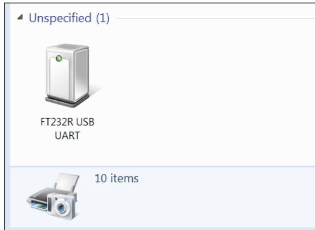
The device is now available to communicate via the IEEE 802.15.4 wireless interface. We could set up a full ZigBee-compliant network, but we're just going to communicate from one device to another directly. So, we'll just use the device as a serial port connection. Double-click on the device and then select the **Hardware** tab; you should see the following screenshot:
