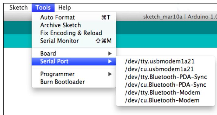
Select the option that begins with **tty.usbmodem**. You may need to remove Arduino to see if you have other devices connected to the port and how this selection changes to identify which port is connected to Arduino. You'll then be connected to the device. You should now be able to open the Blink example, run the code, and see the orange LED flash.
