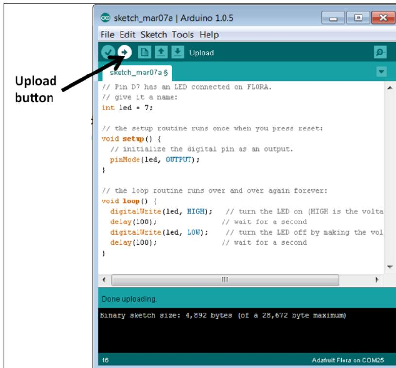
When you have uploaded the file, you should get an indication in the lower-left corner of the IDE. Now the red LED should be flashing much faster. You can change the `delay(1000)` value and see different flash timing.
