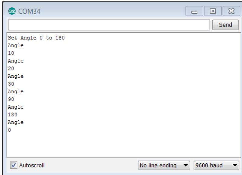
Now you can imagine adding a whole set of servos, one controlled by a different digital output pin on Arduino. However, Arduino itself will soon run out of the ability to supply enough current to control more servos. So if you have projects that require more than just one or two servos, you'll probably want to go with a servo motor shield.
