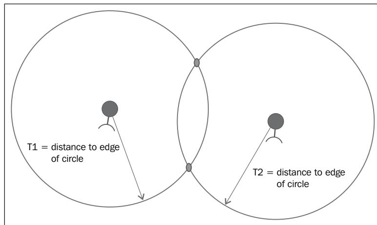
However, since you know that you can only be at points on the circle, you must be at one of the two points that are on both circles. Adding an additional satellite would eliminate one of these two points, thus providing you with an exact location. You need more satellites if you are going to do this in all three dimensions.
