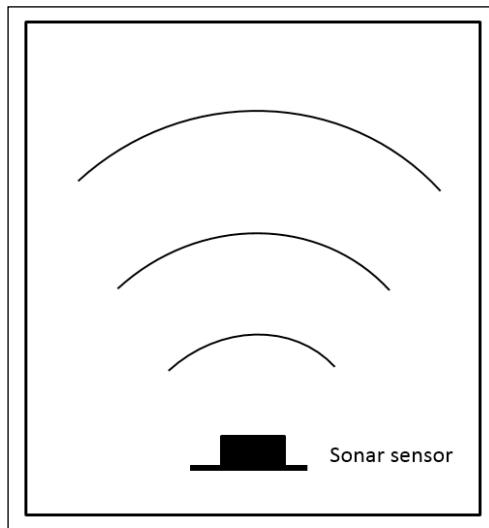
The device sends out a sound wave 10 times a second. If an object is in the path of these waves, the waves reflect off the object. This then returns sound waves to the sensor, as shown in the following diagram:
