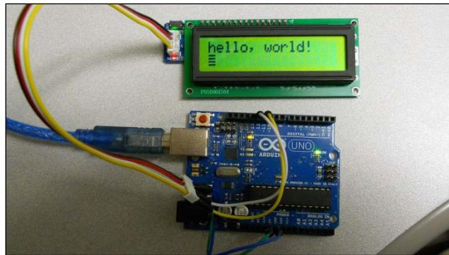
Now, you can add all sorts of text by simply editing the `slcd.print("hello, world!");` line in the `setup()` function or adding this same function to the `loop()` function. Make sure that if you place a message in the loop, use the `delay(2000)` function after it to give the user some time to read the display before you change it.
