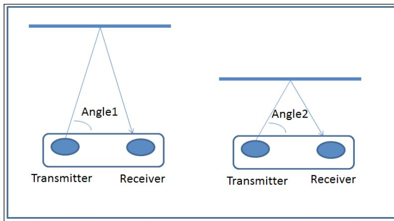
The different angles give you an indication of the distance to the object. Unfortunately, the relationship between the output of the sensor and the distance is not linear, so you'll need to do some calibration to predict the actual distance and its relationship to the output of the sensor. This will be discussed later in this chapter.
