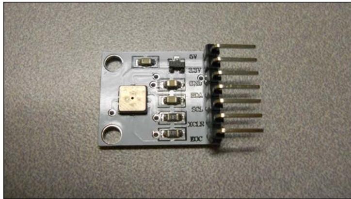
It looks very similar to the digital compass, and just like the earlier two devices, it connects via the I2C interface. You can even use the same libraries you just downloaded for the accelerometer/gyro for I2C support.
