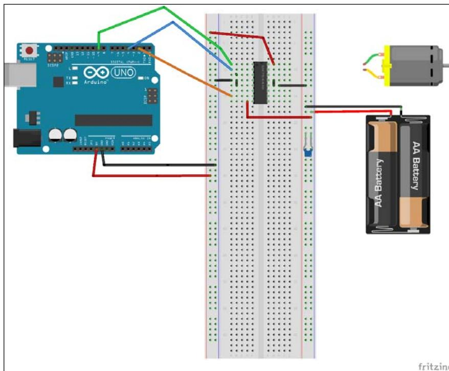
The following table shows Arduino and H-bridge pins and you should connect the pins on Arduino to the pins on the H-bridge:
