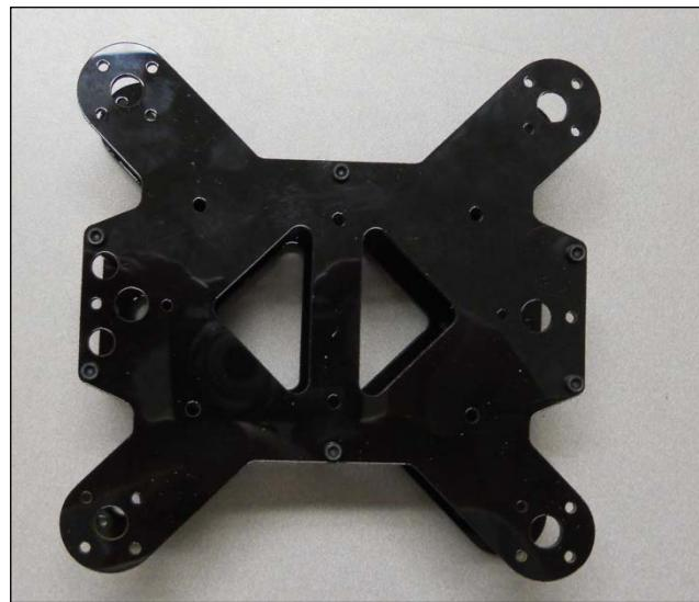
4. And then connect each leg to the body kit. The important part of this step is to make sure you use a bearing on the underside connection of the leg, as shown in the following figure:
