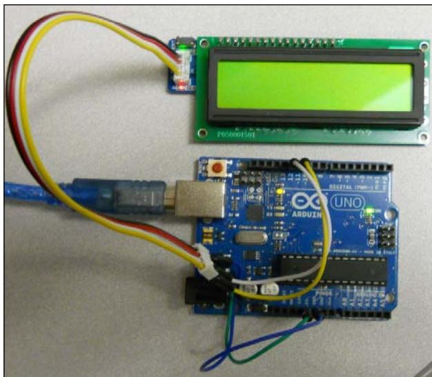
This should complete the hardware connections to the board. You should see the green and red LEDs on the display. This particular type of communication connection is a simple serial connection. The data will be transmitted onto the two pins that you will select in a serial fashion. The display will then take this serial data and translate it to the electrical drive signals needed for the display.
