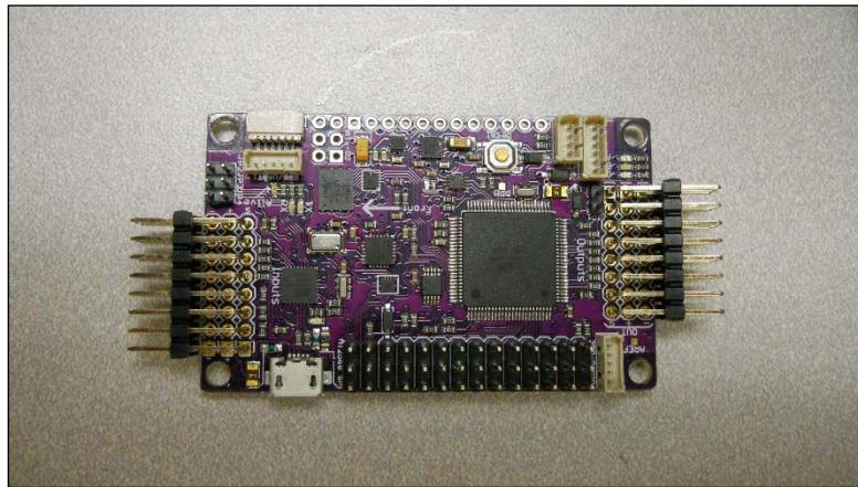
This flight system uses a flight version of Arduino to do the low-level feedback control we talked about earlier. The advantage to this system is that you won't need to create and debug lots of Arduino kit.
