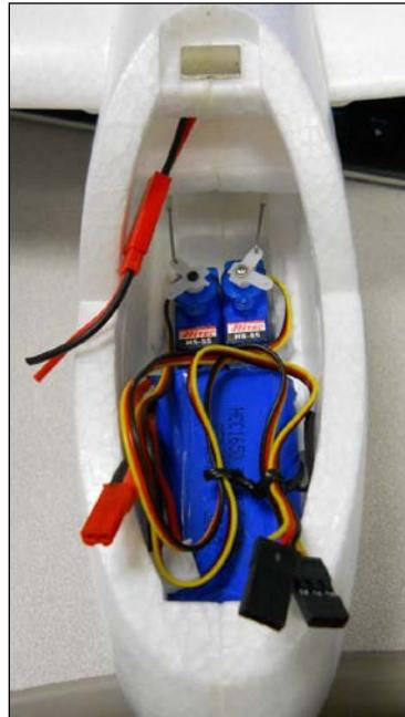
You'll need to connect the two servos, the red and black wires from the motor, and the red and black wires from the battery to your Arduino. The control signals you'll need to provide with your Arduino are the two servos for the control surfaces, and the DC motor that is attached to your propeller is the control for speed.
