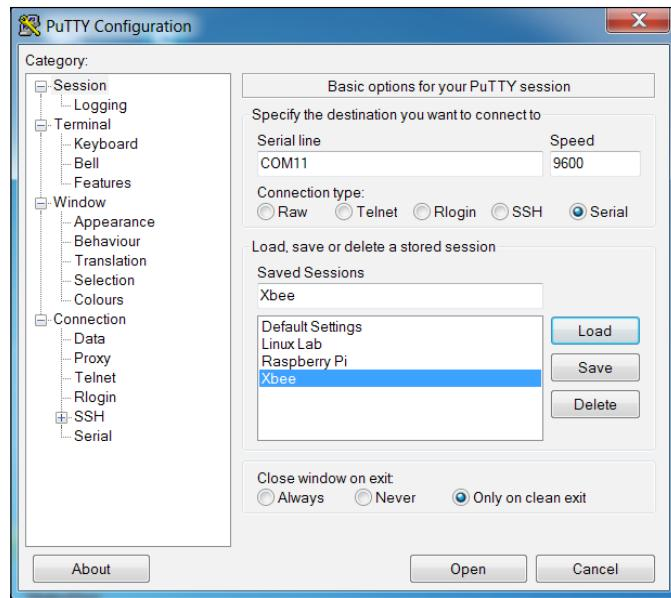
Now, open the terminal window. You should now be able to type 1 and the LED on the remote Arduino will turn on. Typing 0 should turn off the LED. Your PuTTY window should look like the following screenshot if you select **Force on** in the **Local echo** option and if the **Implicit CR in every LF** and **Implicit LF in every CR** options are checked:
