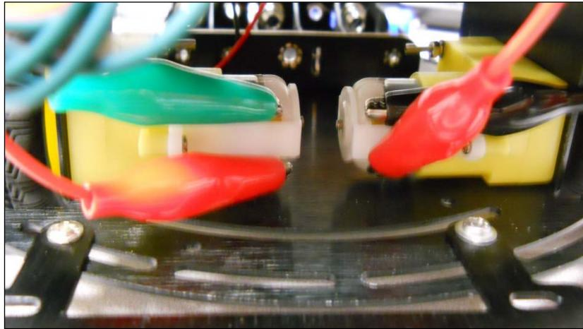
The final step is to connect the alligator clip wires to the motor controller shield. I did this with the male-to-male solderless jumper wires. First, insert the cables into the motor shield screw connectors. There are two sets of connections—one for each motor. Then, attach the alligator clips to the other ends of these wires as shown in the following figure:
