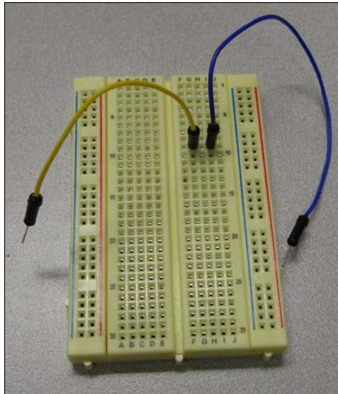
The two rows on each side of the board are generally designed to provide power, so they are connected up and down.
