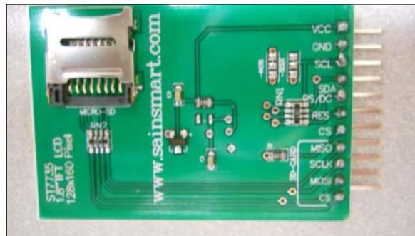
2. This display uses the SPI interface, so you'll be connecting to the top seven pins shown here. The SPI interface is a serial interface but is synchronous, so it provides a more robust communication path. Here is the wiring table that shows which pins to connect to between your Arduino and the display:
