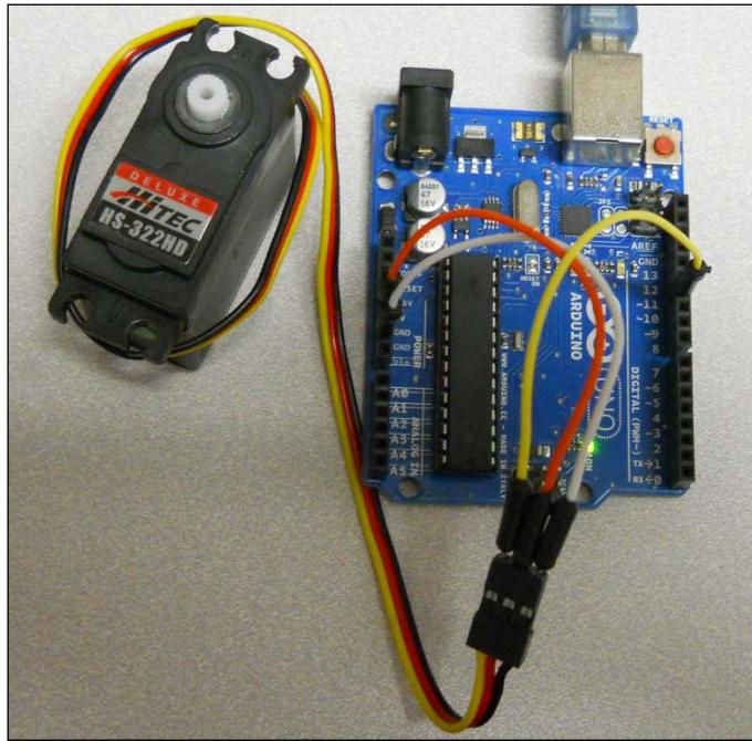
Just a word of caution, this works well with a single servo; you will not want to use the method for more than just one or two servos. Now that you have made these connections, you are ready to write the code to make your servo move.
