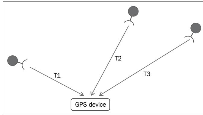
The GPS device is able to detect the three signals and the time delays associated with receiving these signals.
