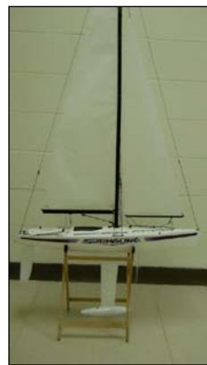
This sailboat is ready to sail via radio control. This means that it has two servos mounted inside: one to control the sail and the other to control the rudder. The following is an image of these two servos that are connected to the sail and rudder:
