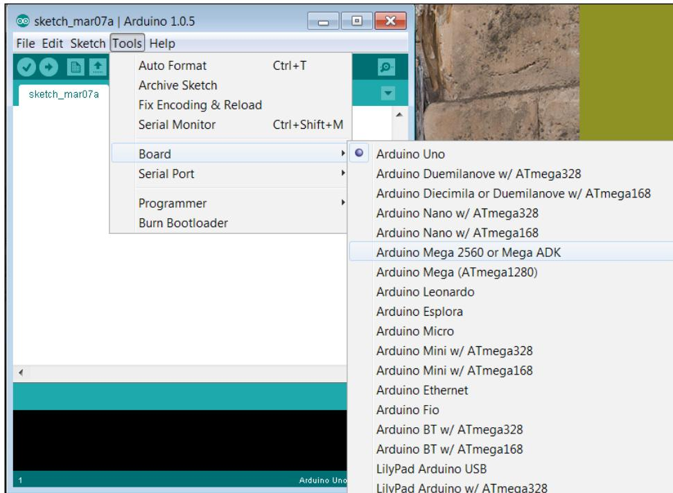
If you have a different COM port number, make sure you set that by navigating to **Tools | Serial Port**. You can now upload the Blink code, and the orange LED should be blinking on Mega.
