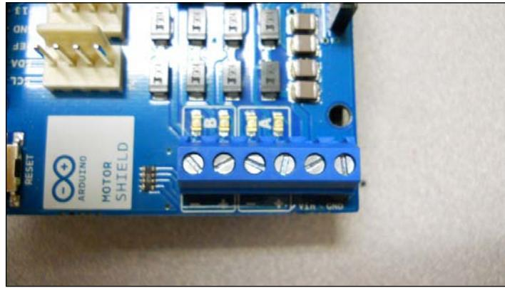
It is these three connections that you will use in this example. First, however, place the board on top of Arduino, in the same way that you placed the display shield from the example in *Chapter 5, Working with Displays*. Then, mount the two boards to the top of your two-wheeled robotic platform, as shown in the following figure:
