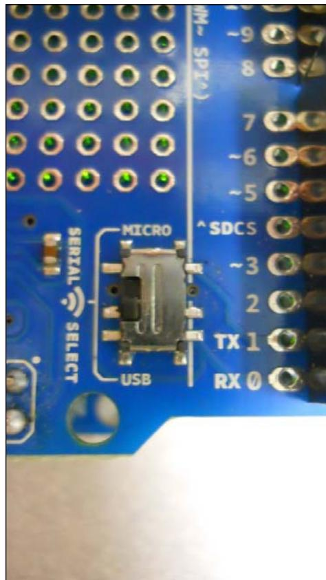
When you are programming the device, you'll want this switch to be in the USB location. When you are ready to communicate with the device, you'll want to switch this to the MICRO setting. So, change it to the MICRO setting once your sketch has finished compiling and uploading to Arduino. Then, connect your Arduino to a battery.
