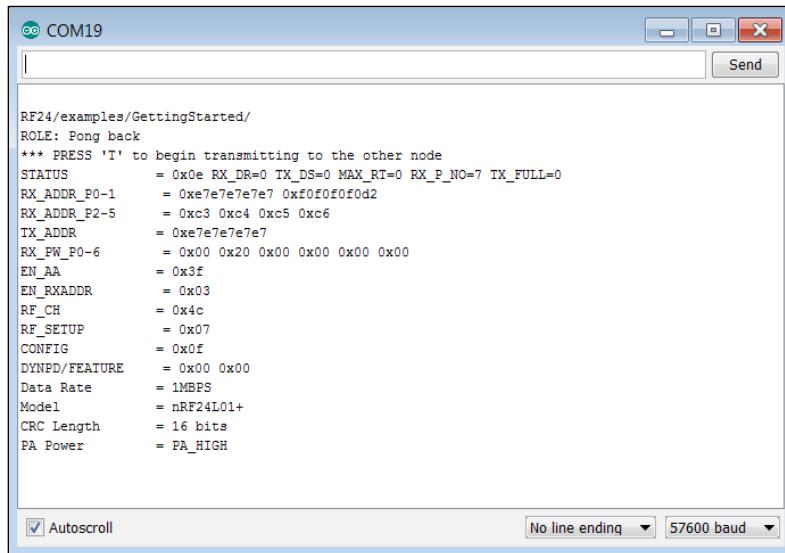
This shows the configuration of the first device. If you receive 0 for all values, you probably have your device connected incorrectly. Initially, this first device will be in receive mode, listening for a message, and when it receives one, it will send this message back to the sender.
