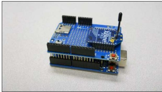
Now, let's start to configure your two devices to talk. You'll need to configure both devices by plugging them into your host computer. Plug one of the devices into the small XBee-specific USB shield and then connect the shield to your personal computer. Your computer should find the latest drivers for the device. You should see your device when you select the **Devices and Printers** selection from the **Start** menu, as shown in the following screenshot:
