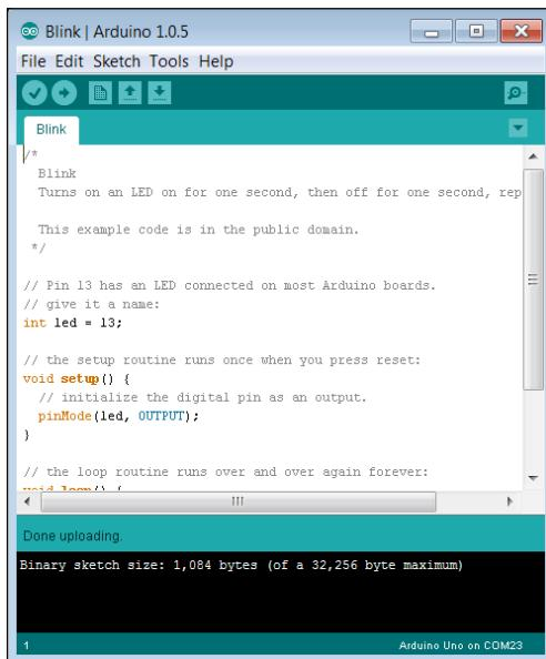
5. When the program is uploaded, it will automatically start running and the orange LED on the Arduino Uno will blink:
