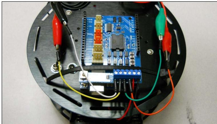
Insert some batteries, and then connect Arduino to the computer via the USB cable. Now, you are ready to start programming to control the motors.
