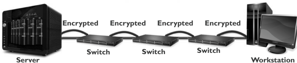
Figure 6-18 MACSec provides layer 2 frame protection.
