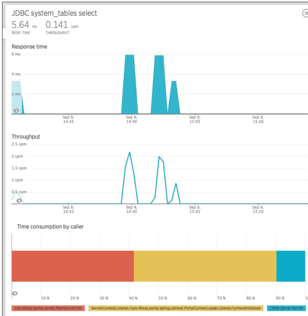
This gives you a breakdown of that particular transaction and highlights the response over time alongside throughput. Of particular interest is the bottom graph; this illustrates the most common transactions that are calling this an SQL query, charted by the overall time spent being called by that particular transaction. These are linked to the transaction view; thus, allowing you to see detailed information about that particular transaction.
