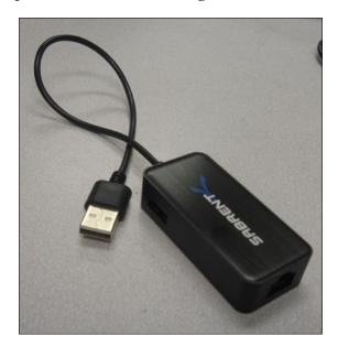
Connecting the Raspberry Pi Zero in this way is actually amazingly easy. Simply plug the USB to LAN adapter into the powered USB hub, connect an active LAN cable and you should then have Internet access.
