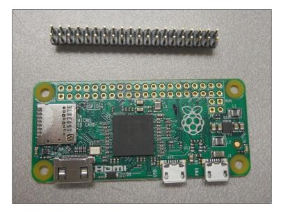
Note that the GPIO pin male headers are not pre-soldered to the board; you'll want to do that. You can buy these at most online electronics retailers. You should also become familiar with the various connections on the board. Here, you can see the Raspberry Pi Zero with the connector soldered and the connections labeled for your information:
