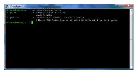
There are two possible audio devices that you can use. The first is the internal Raspberry Pi audio, which is connected to the audio port, and the second is the USB audio plugin. You could use the USB audio plugin to record the sound and the Raspberry Pi for the audio output to play the sound, though it is easier to just use the USB audio plugin to create and record sound.
