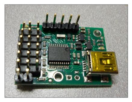
Make sure you order the assembled version. This piece of hardware will turn the USB commands from the Raspberry Pi Zero into signals that control your servo motors. There are two connections that you'll need to make to the servo controller to get started: the first to the servo motors and the second to a power source.
