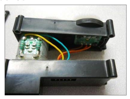
As you can see in the preceding image, the blue and yellow wires are attached to a DC motor, and the orange, brown, and red wires are attached to another control circuit. The motor will drive the wheels left or right, the polarity of the voltage will determine the direction, and its magnitude will cause the wheels to turn more or less sharply. The orange, brown, and red wires are interesting, as their purpose is a bit difficult to discover.
