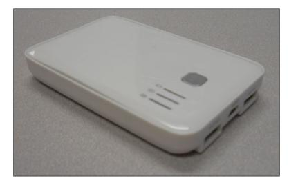
In both cases, make sure that the unit can supply enough current. You'll need a supply that can provide at least 1000 mA at 5 volts. There are two USB charge connections on this battery which makes it easy to plug the Raspberry Pi Zero into one and the powered USB hub into the other. Do not plug in the board just yet, you first need to connect the rest of the hardware and configure the microSD card. However, you are now ready to connect the rest of the hardware.
