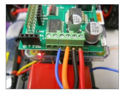
2. Next, connect the rear drive signal to the motor 1 connectors on the board, as in the following image:
