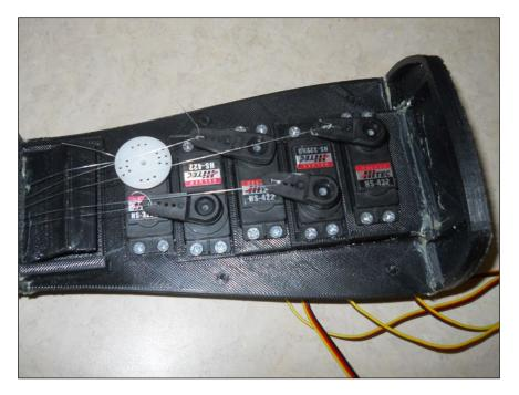
Here is an image of how to connect the fishing lines to a servo:
