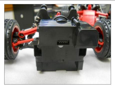
The five-pin connector that comes from the control module is shown in the following image:
