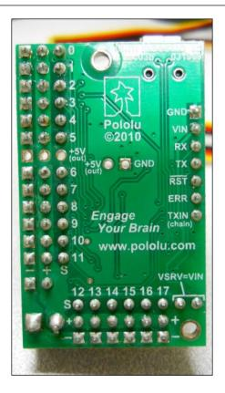
Now you need to connect the servo motor controller to your battery. For this project, you can use a 2S RC LiPo battery. The 2S means that the battery will have two cells, with an output voltage of 7.2 volts. It will supply the voltage and current needed by your servos, which can be in the order of 2 amps, as shown in the following image:
