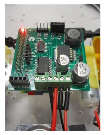
2. Next, connect one of the drive signals to the motor 1 connector on the board. Connect motor 1 to the right motor and motor 2 to the left, as shown:
