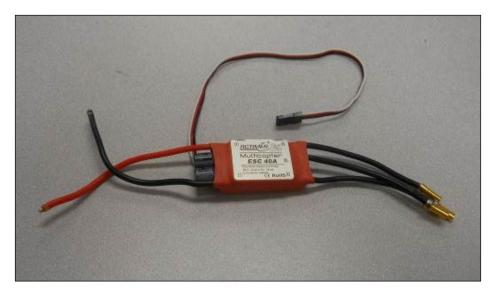
The red and black wire connectors are the connectors that are soldered to the bottom plate of the frame. The other three connectors will connect to the motor.
