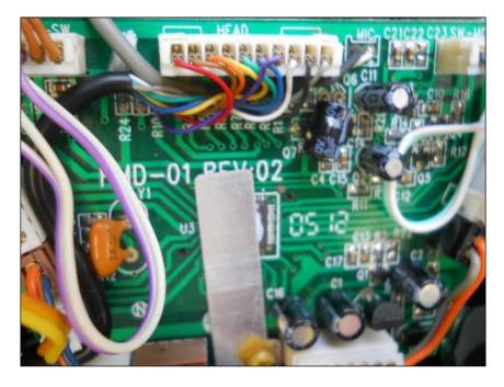
There are only two wires that you are interested in. The first is the black wire, which is the GND for the Robosapien system. The second is the white wire. This is the serial connection that controls the command for the Robosapien.
