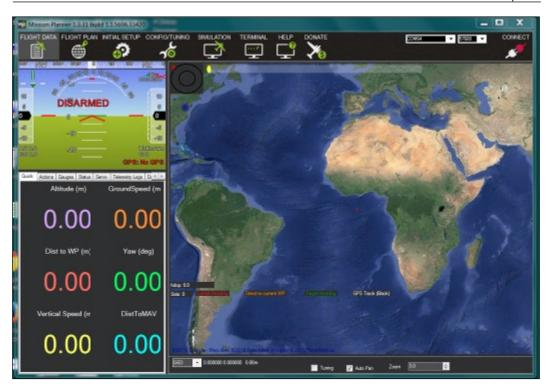
This is the basic screen. You'll then need to configure your radio's COM port and then press the **CONNECT** button in the corner on the upper right-hand side of the screen. As you move the quadcopter around, you will see the measurements change. If you are having problems connecting to the Pixhawk, there is lot of help available on the website.
