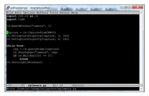
The two lines that you'll add are the two with the cv.SetCaptureProperty; they will set the resolution of the image to 360 by 240. To run this program, you'll need to either have a display and keyboard connected to Raspberry Pi or use vncviewer. When you run the code, you should see the window displayed as shown:
