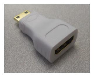
To use this connector, simply connect the adapter to your Raspberry Pi Zero, then the cable with the regular HDMI connections to the adapter and your TV or monitor that has an HDMI input connector. HDMI monitors are relatively new but if you have a monitor that has a DVI input, you can buy relatively inexpensive adapters that provide an interface between DVI and HDMI.
