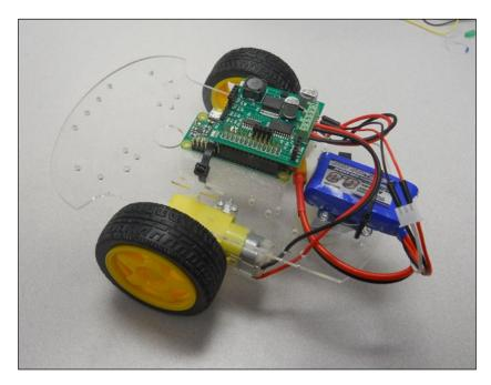
3. Then, connect the second drive connector to the motor 2 connector on the board. The entire set of connections should look like this:
