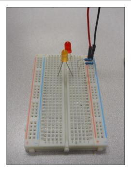
Now you'll use the jumper wires to connect to Raspberry Pi Zero's GPIO pins. You'll connect to pin 13 (GPIO 27) and pin 15 (GPIO 22), as shown:
