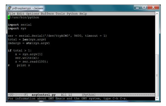
To run this program, type python argControl.py f and the robot will respond to that command. To make this program executable without the Python command, type chmod +x argControl.py and you will be able to run the program by typing ./argControl.py f. You'll need this later when you want to run this program from your voice control program.
