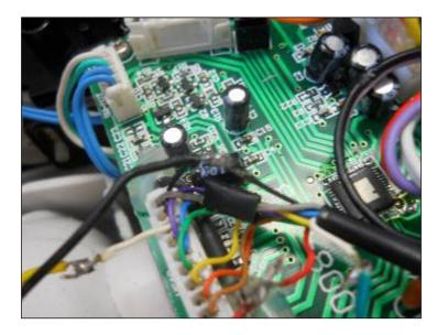
3. Now, snip the white wire and connect a wire to the end that is connected to the white header connector, as shown in this image:
