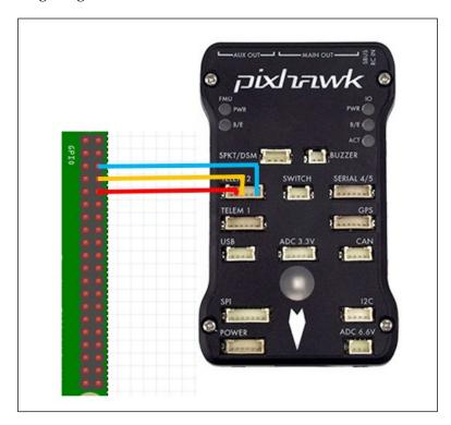
Now that this is connected, you can access the Pixhawk from Raspberry Pi Zero using the MAVLink. You'll need to add and configure the Raspberry Pi Zero to complete the connection. To do this, run raspi-config and choose the **8** Advanced Options, Configure advanced settings option, as shown in the following screenshot:
