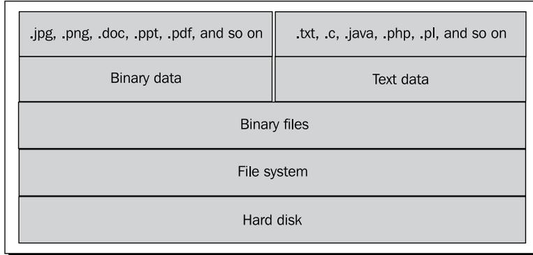
Going from the top to the bottom, it is a layered approach starting with how a user sees a file, how a computer sees it, until its storage at the bottommost layer.
