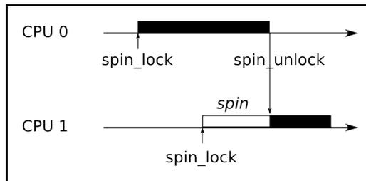
The thread that holds the spin lock cannot be preempted since doing so may make the new thread enter the same code and deadlock when it tries to lock the same spin lock. Consequently, in mainline Linux, locking a spin lock disables kernel preemption, creating an atomic context. This means that a low priority thread that holds a spin lock can prevent a high-priority thread from being scheduled.
