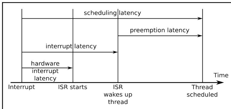
Firstly, there is the hardware interrupt latency from the point at which an interrupt is asserted until the **interrupt service routine (ISR)** begins to run. A small part of this is the delay in the interrupt hardware itself, but the biggest problem is due to interrupts being disabled in software. Minimizing this *IRQ off time* is important.
