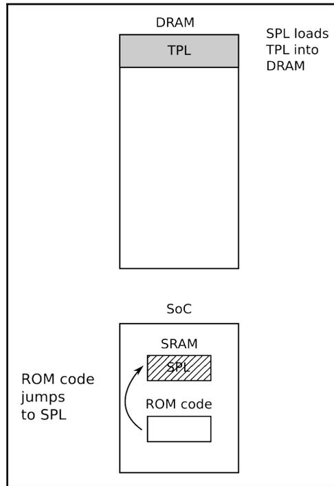
The SPL may be open source, as is the case with the TI x-loader and Atmel AT91Bootstrap, but it is quite common for it to contain proprietary code that is supplied by the manufacturer as a binary blob.
