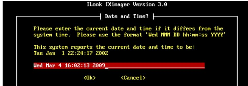
IXImager: reading the computer clock and adding a record of the actual time for comparison during analysis
