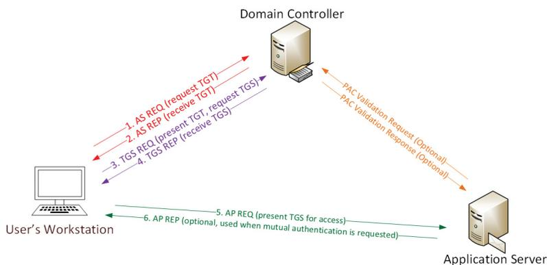
**Figure 7-1:** The KERBEROS authentication process (diagram courtesy of Sean Metcalf and [adsecurity.org](http://adsecurity.org))
