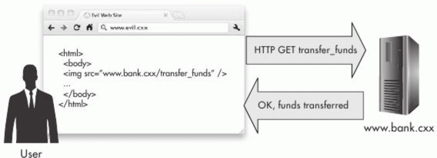
Figure 6-8 A browser automatically makes a malicious request to transfer funds from the user's bank account at www.bank.cxx .
