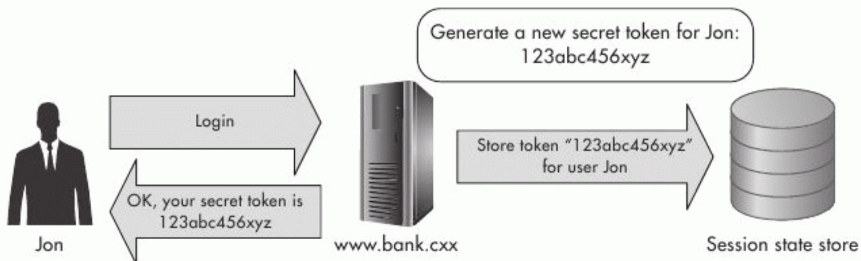
Figure 6-9 A web server generates, stores, and sends back a unique nonce for the user.
