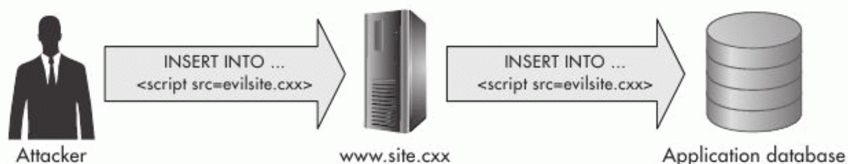
Figure 7-1 An attacker uses SQL injection to insert an HTML link to a malware site.
