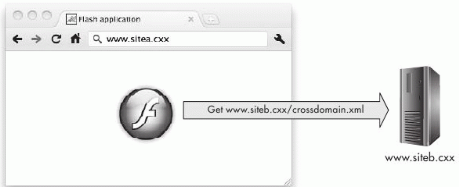
Figure 5-6 The web site www.siteB.cxx uses a Flash cross-domain policy file to allow Flash applications to access it from other origins.
